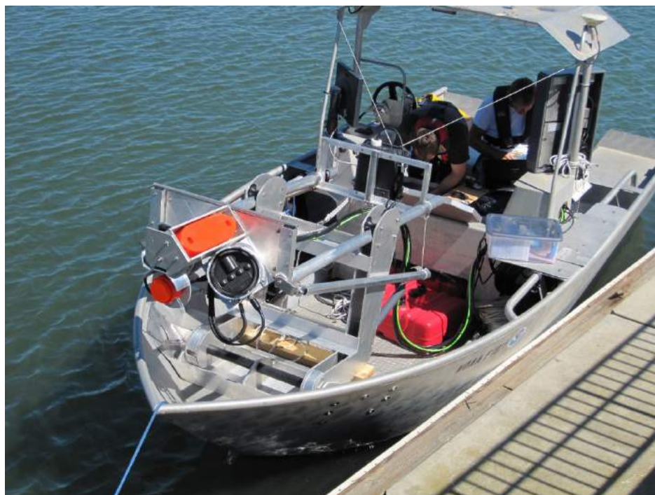
Figure 4-2. A retractable bow mount for deploying a down-projecting 200-kHz split-beam transducer (orange cylinder), side-projecting 120-kHz split-beam transducer (orange boat shape), and two 500-kHz multi-beam transducers (black, only port-side is fully visible). A sensor package mounted on top of the apparatus (black box) provides attitude, heading, heave, position, and velocity information. To deploy, the transducer array is pushed forward, rotated down into the water, and stabilizing struts attach to the gunwale on each side of the bow.
